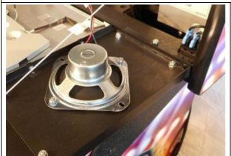
The pro and most premium trims ship with 4" speakers and speaker plates from the factory. This size speaker and plate will not work with PixlWav speaker light kits.
