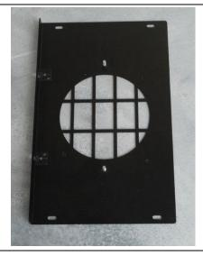
The 4" speaker plate has only two mounting studs for the speaker.
