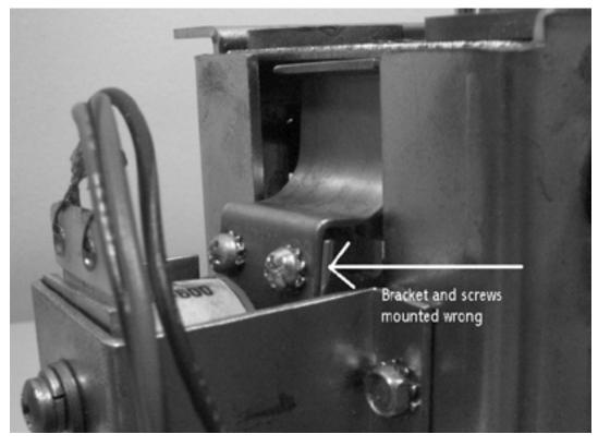
Picture above shows the latch mounted incorrectly.
