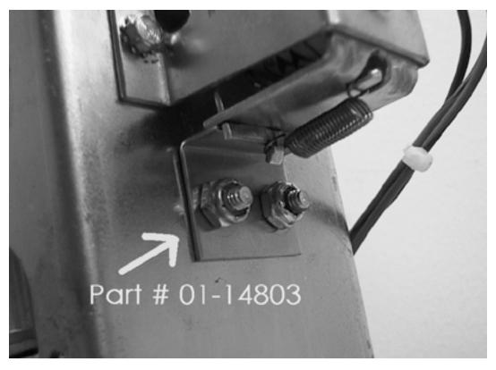
Part #01-14803 prevents the coil frame from bending.
