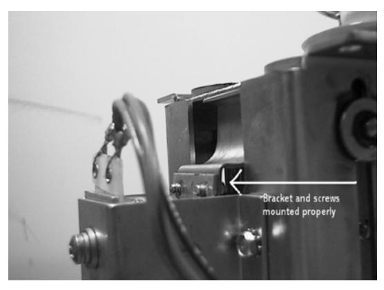
Picture above shows the latch mounted correctly.
